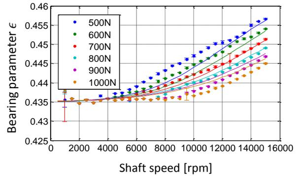
**Figure 11: Changes of the bearing parameter caused by the pre load and the rotation speed**
