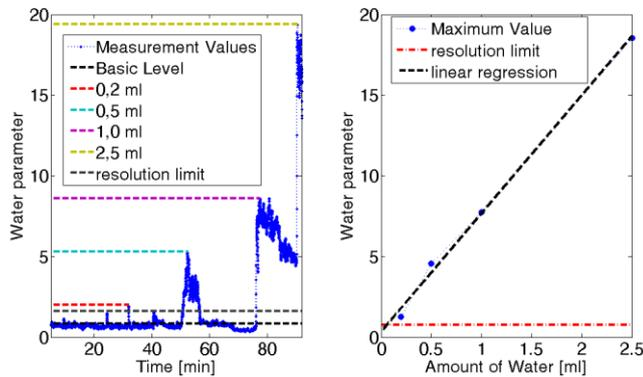
**Figure 10: Water parameter and the behavior by increasing amount of water in an 6306 groove ball bearing**
