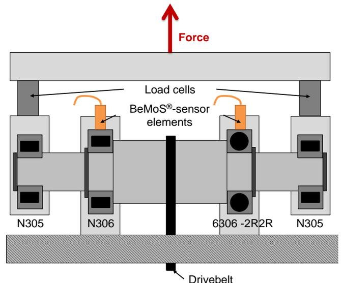
**Figure 5: schematic structure of the test-bench**
