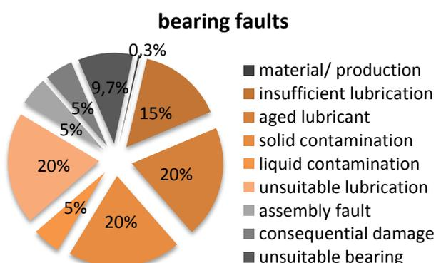
Figure 1: Causes of bearing faults [1]
