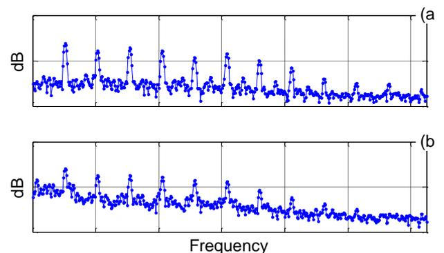
Figure 9: Frequency spectra of pure grease lubrication (a) and water contamination (b)
