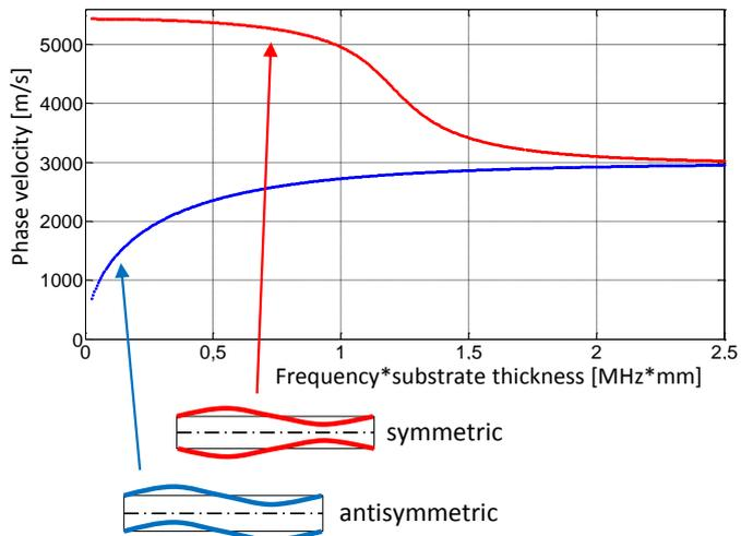
**Figure 3: Phase velocity and displacement of the basic symmetric and antisymmetric modes of steel**
