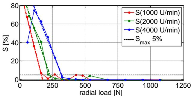
Figure 7: Slip behavior at different operation conditions
