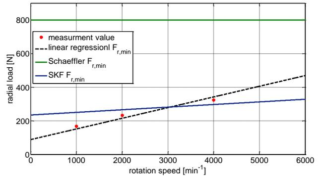
Figure 8: slip measurement results compared to the guidelines from the bearing manufacturer
