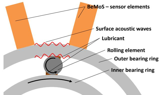
**Figure 4: Mounting of the sensor elements and structure of the transmission line**
