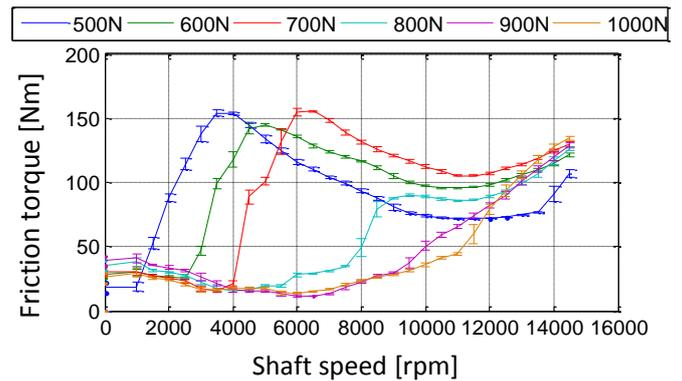
**Figure 12: Measurement of the friction torque in different operation conditions**
