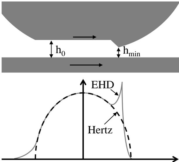
Figure 2: Pressure distribution and lubrication gap geometry in an EHD-contact
